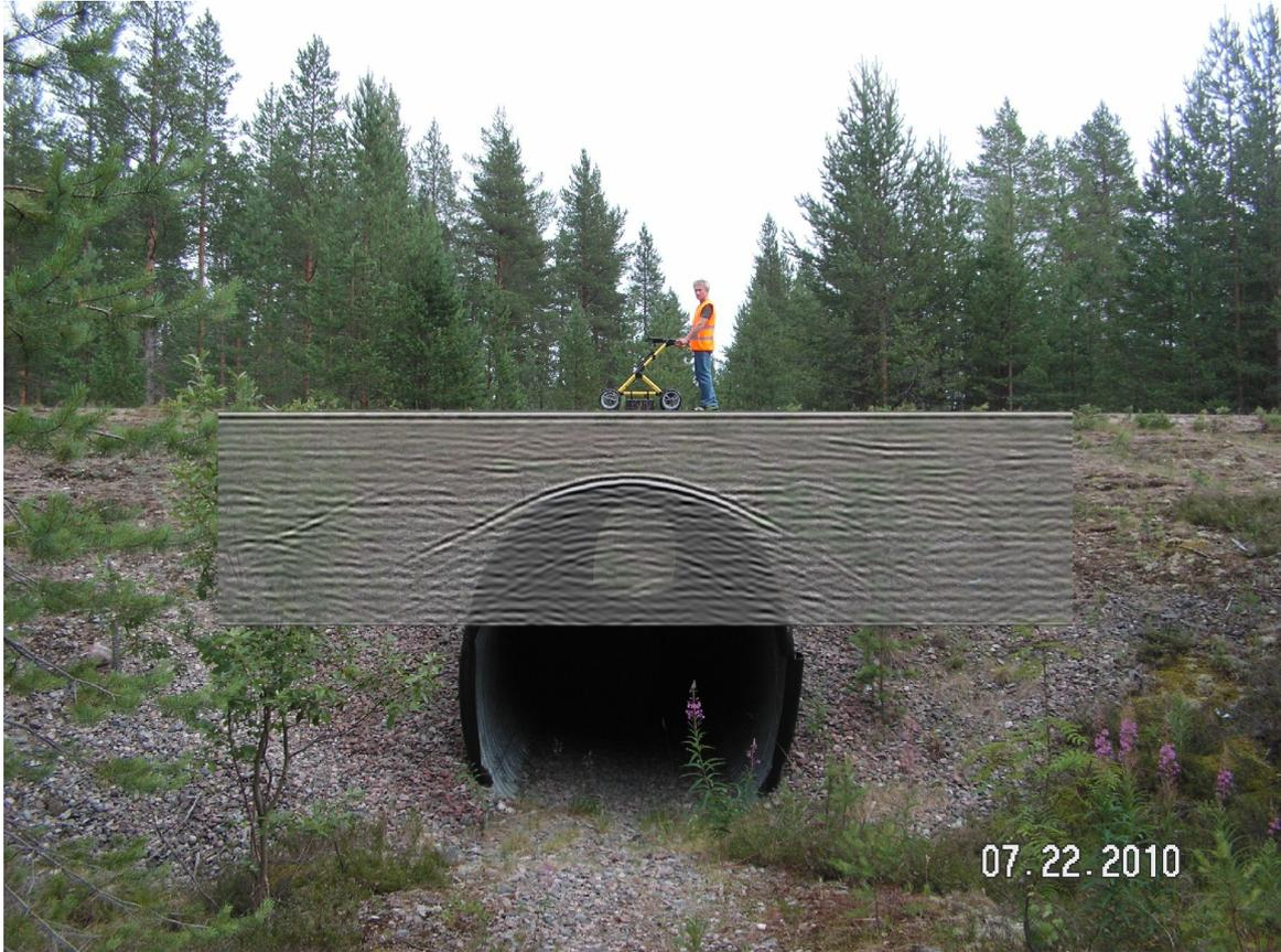
*Fig. 5 Composite picture showing the survey area and the GCB-500 data superimposed.*
