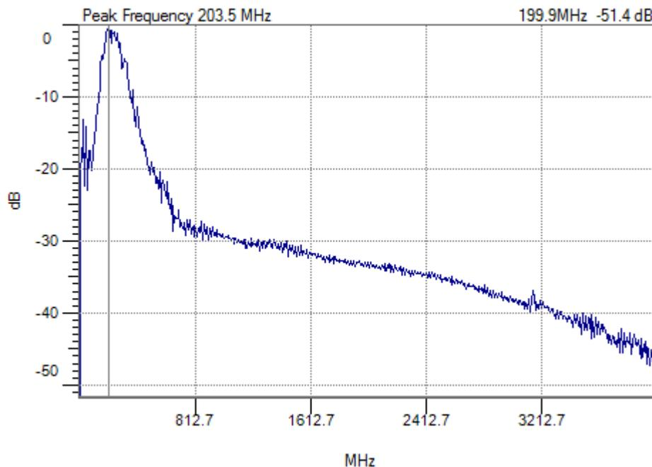
Fig. 1 Power spectrum of the GCB-200 ground coupled antenna.
